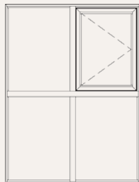
Elevation View: Window Wall with Casement
