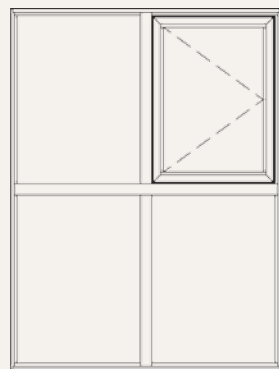
Elevation View: Window Wall with Casement
